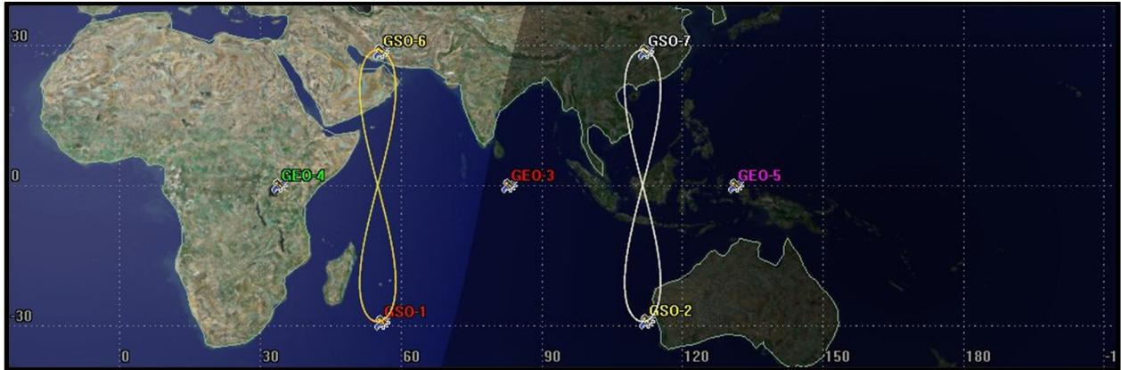
**Fig 1 Indian Regional Navigation Satellite System Schematic (Conceptual)**
