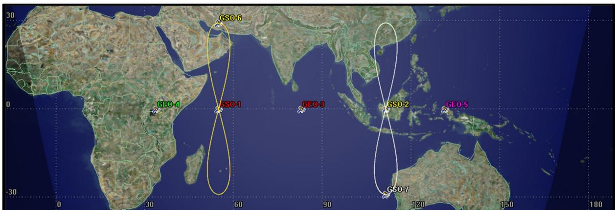
**Fig 4 Geosynchronous satellites positioned for maximum coverage and continuous visibility (north/south of target area)**
