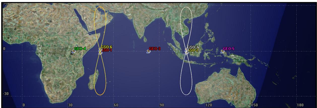
Fig 3 "Satellite Crowding" over the equator (when set apart by  $180^\circ$ )
